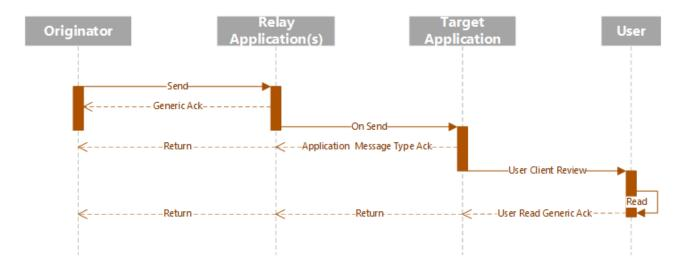
Should delivery fail, faults that can be remedied are highlighted. These would have otherwise been unknown to the sender as the receiver would be unaware they should have received a message. This also allows systems to provide notification of human read acknowledgements of messages, mapping the sending application to the provider viewing the message contents.
